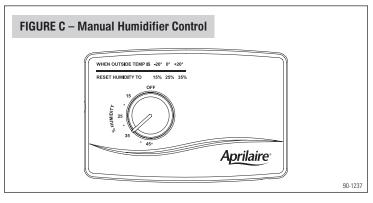
Your Aprilaire humidifier is controlled by a Manual Humidifier Control (see **Figure C**). The Manual Humidifier Control is installed either in the cold air return duct or on an interior wall of the home. With the Manual Humidifier Control, it is important to anticipate a drop in outdoor temperature and reduce the setting accordingly to avoid excessive condensation, just as with the Automatic Digital Humidifier Control installed in Manual Mode (see page 6).
