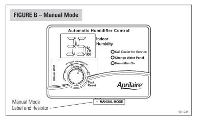
When installed in the Manual Mode (see **Figure B**), it is important to anticipate a drop in outdoor temperature and reduce the setting accordingly to avoid excessive condensation. For example, with an outdoor temperature of 20°F the correct setting will be 35% RH. If the temperature is expected to fall to 0°F that evening, then merely reduce the setting to 25% several hours prior to the temperature change.
