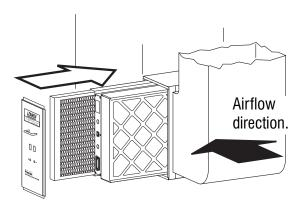
**Fig. 4** Slide PCO-12C/20C assembly with provided pleated filter and metal insert into the PCO-12C/20C cabinet.
