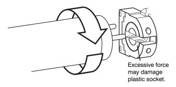
Fig.2 Verify proper installation of lamps.
