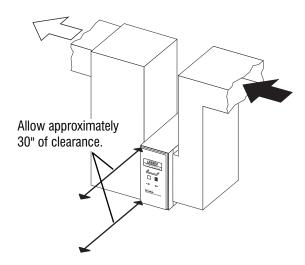
Fig.3 Install PCO-12C/20C in the return air duct.
