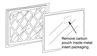
**Fig. 1** Remove and discard all wrapping and packaging material prior to installation and operation of PCO-12C/20C.
